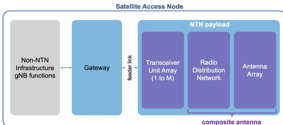
Figure 1: 3GPP NR Satellite Access Node (SAN).
