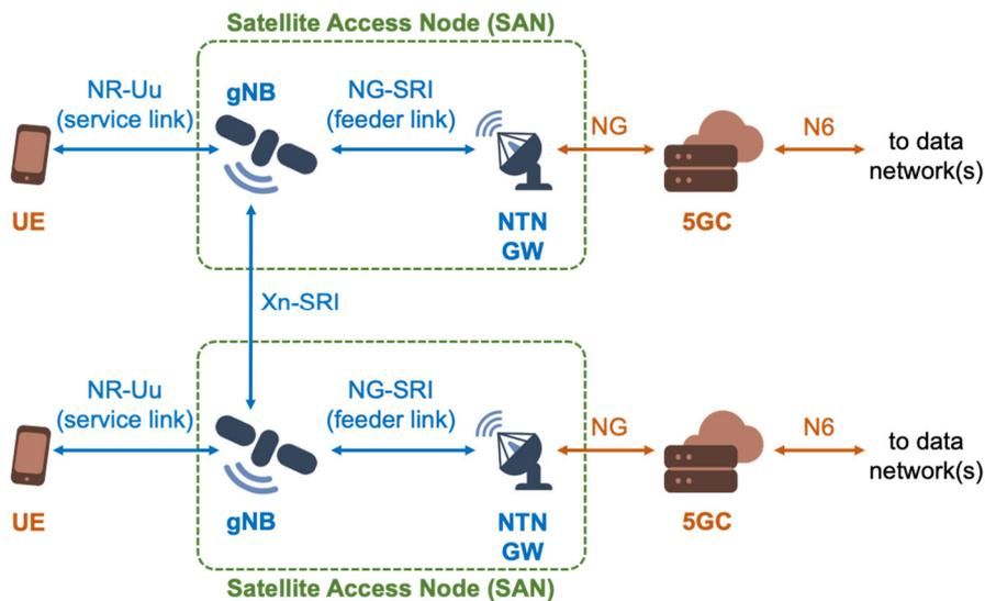
Figure 9: NTN architecture with regenerative payload and direct access: full gNB on-board with ISL.
