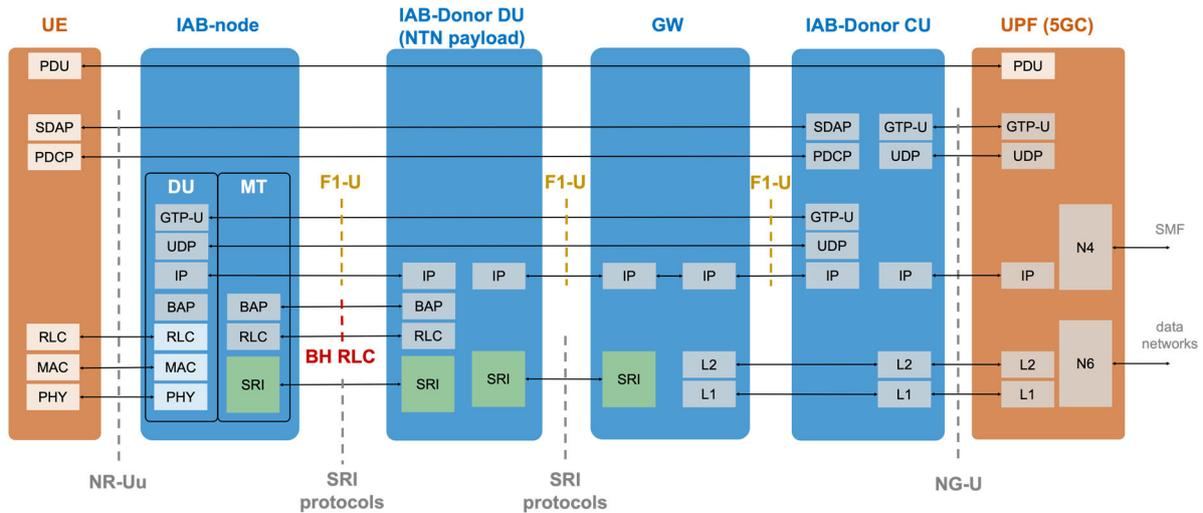
Figure 24: UP protocol stack: NTN architecture for indirect access with regenerative payload, with IAB-Donor DU on-board.
