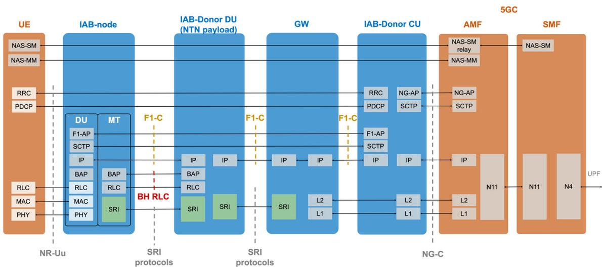
Figure 25: CP protocol stack: NTN architecture for indirect access with regenerative payload, with IAB-Donor DU on-board.
