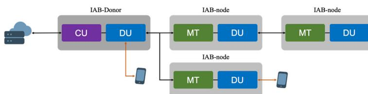
Figure 15: Hierarchical RAN structure based on IAB nodes.
