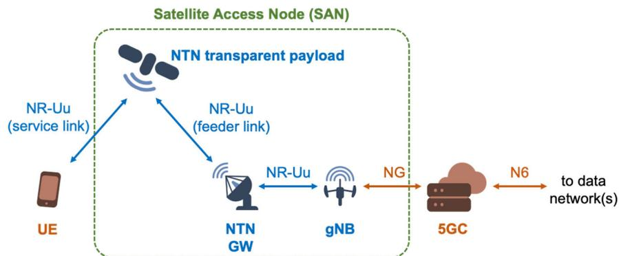
Figure 2: NTN architecture with transparent payload and direct access.
