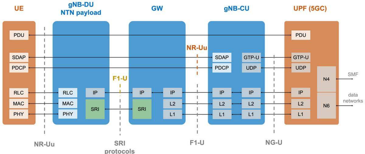
Figure 13: UP protocol stack: regenerative payload with functional split for direct access.
