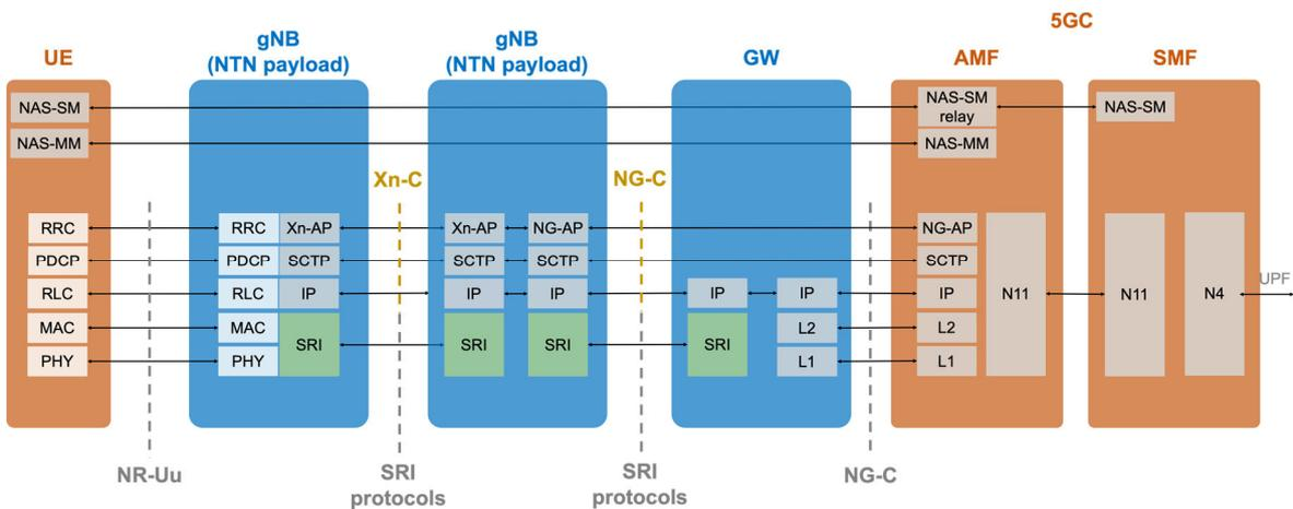
Figure 11: CP protocol stack: regenerative payload and direct access with full gNB on-board and ISL.
