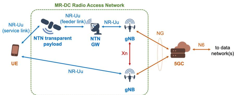
Figure 28: MR-DC architecture between TN and NTN with transparent payload.
