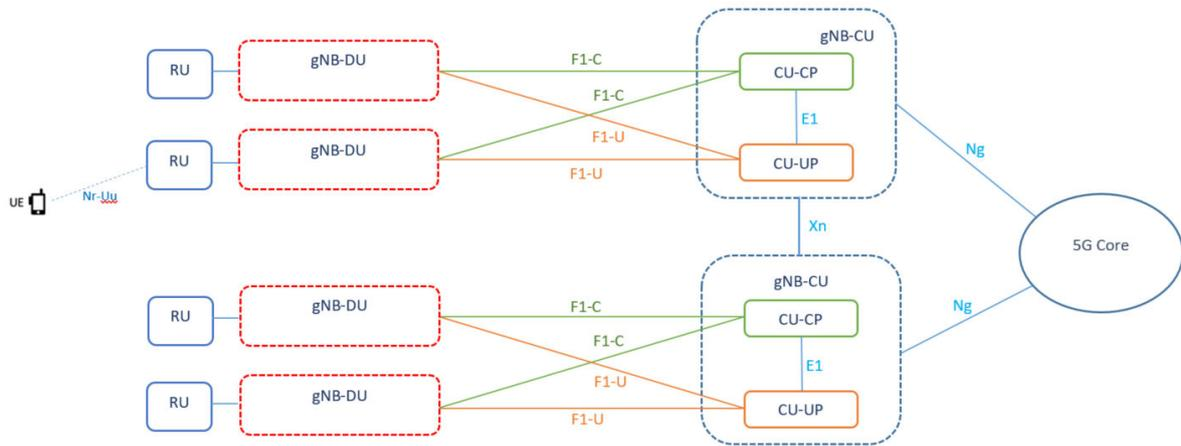
Figure 39: High-level architecture of a standard TN.
