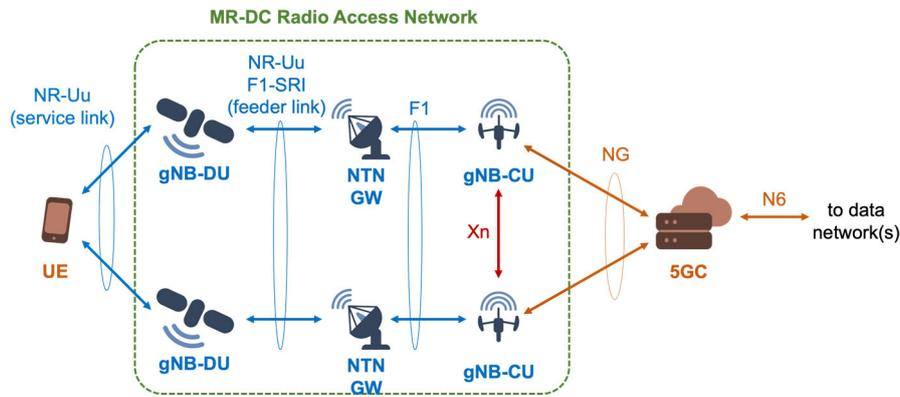
Figure 33: MR-DC architecture between NTN and NTN with regenerative payload: gNB-DU on-board.
