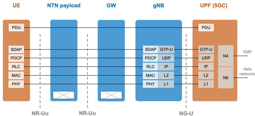
Figure 3: UP protocol stack: transparent payload and direct access.
