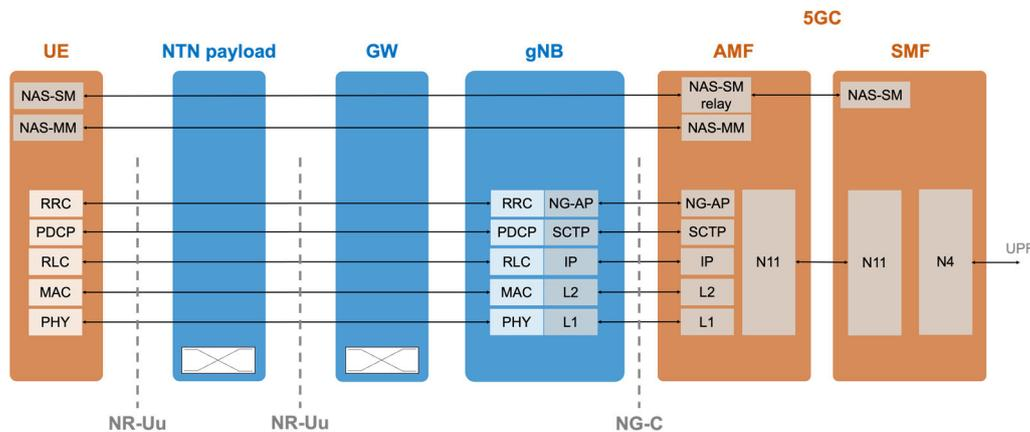
Figure 4: CP protocol stack: transparent payload and direct access.
