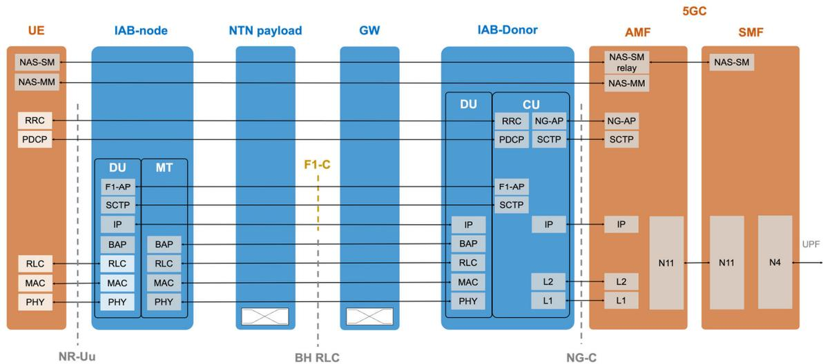
Figure 18: CP protocol stack: NTN architecture for indirect access with transparent payload, with backhaul to the IAB-Donor.
