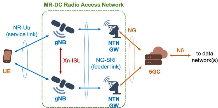
Figure 31: MR-DC architecture between NTN and NTN with regenerative payload: full gNB on-board.
