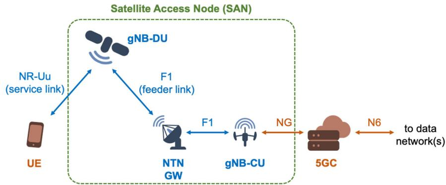
Figure 12: NTN architecture for direct access with regenerative payload and functional split.
