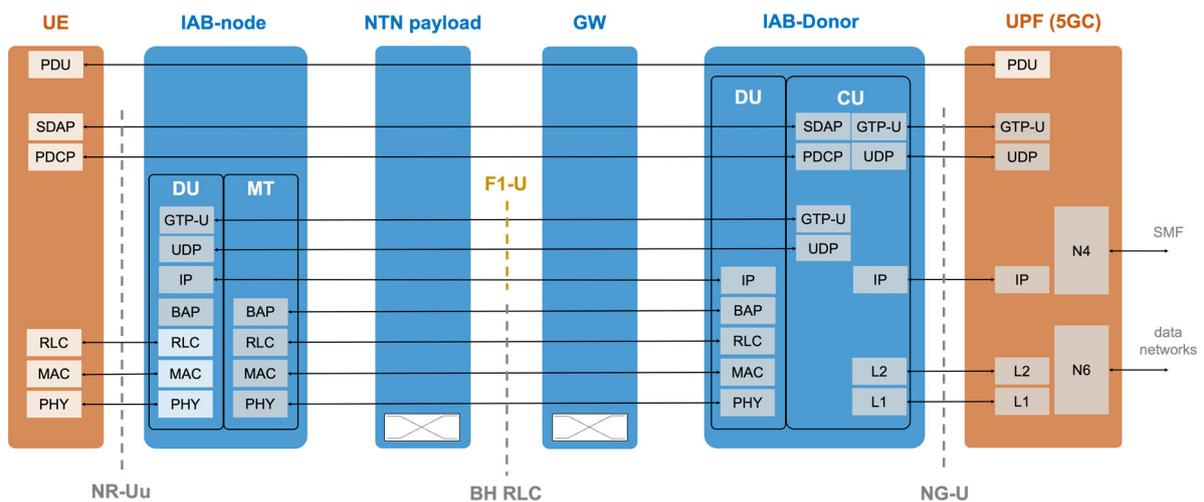
Figure 17: UP protocol stack: NTN architecture for indirect access with transparent payload, with backhaul to the IAB-Donor.
