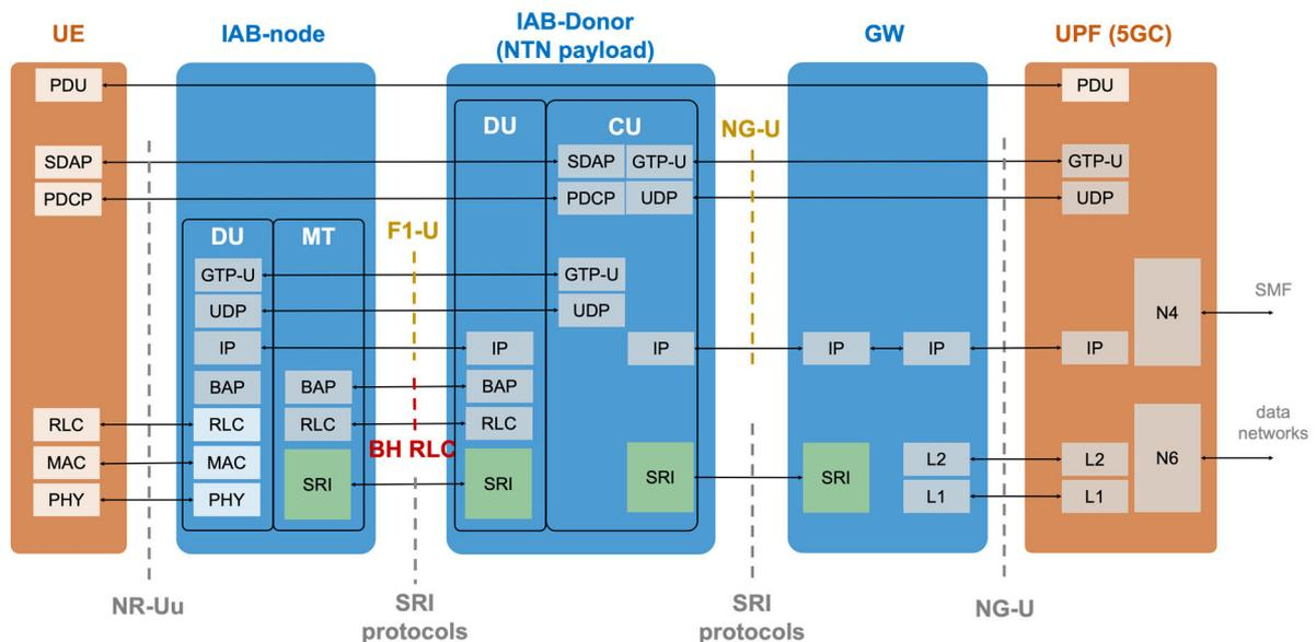
Figure 21: UP protocol stack: NTN architecture for indirect access with regenerative payload, with full IAB-Donor on-board.
