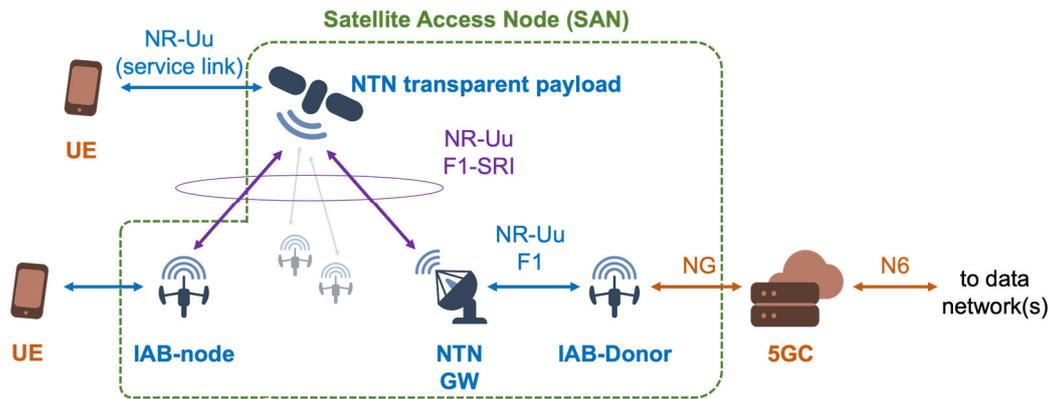
Figure 16: NTN architecture for indirect access with transparent payload: backhaul to the IAB-Donor.
