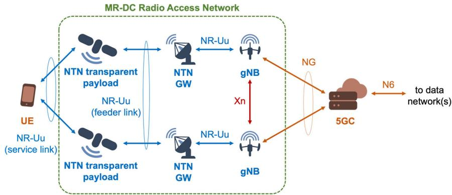
Figure 29: MR-DC architecture between NTN and NTN with transparent payload.
