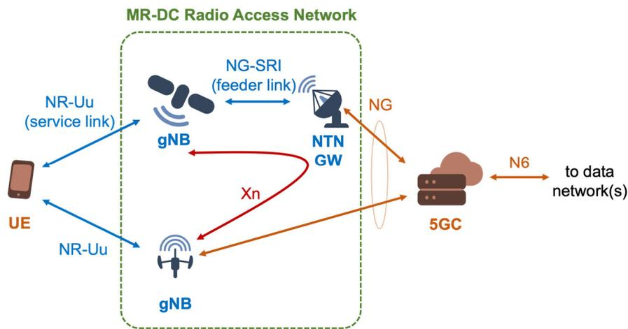
Figure 30: MR-DC architecture between TN and NTN with regenerative payload: full gNB on-board.
