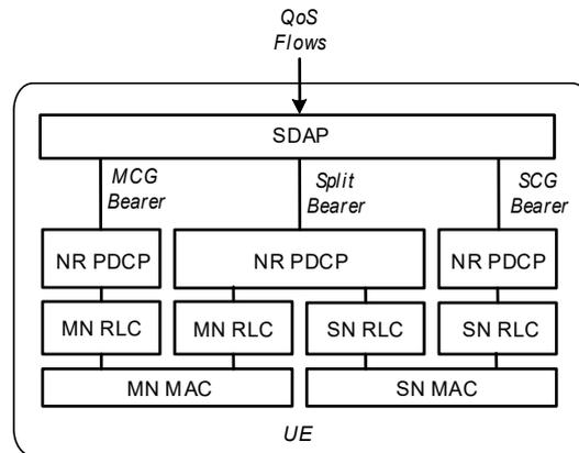
Figure 26: Radio protocol architecture for MCG, SCG, and split bearers for the UE in NR-MC, [17].
