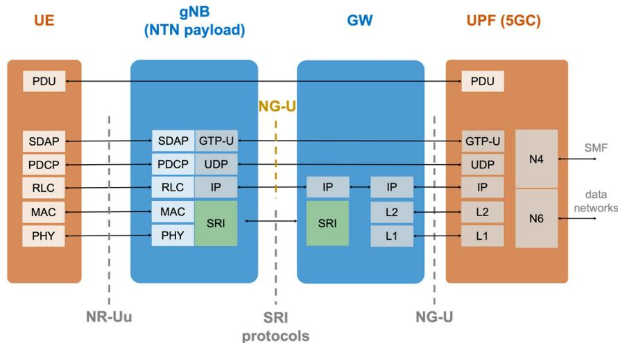
Figure 7: UP protocol stack: regenerative payload and direct access with full gNB on-board.
