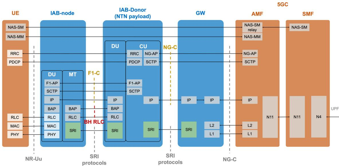
Figure 22: CP protocol stack: NTN architecture for indirect access with regenerative payload, with full IAB-Donor on-board.
