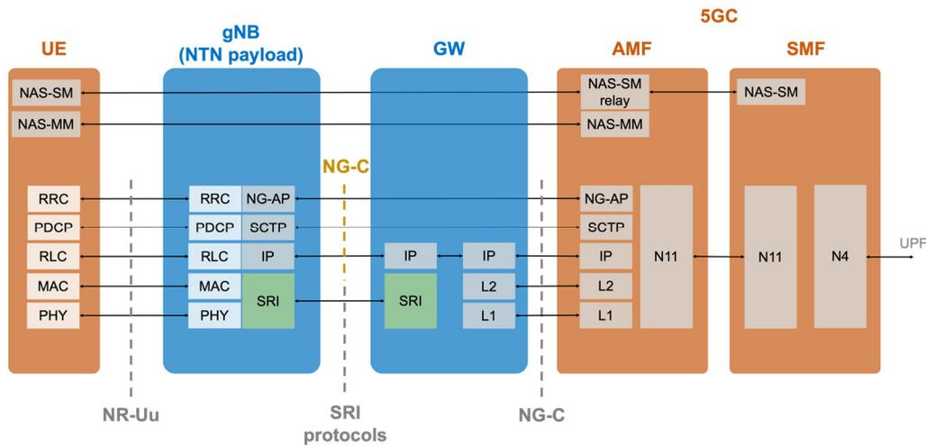
Figure 8: CP protocol stack: regenerative payload and direct access with full gNB on-board.
