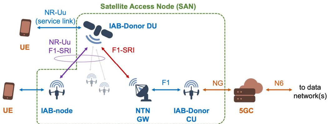
Figure 23: NTN architecture for indirect access with regenerative payload: IAB-Donor DU on-board.
