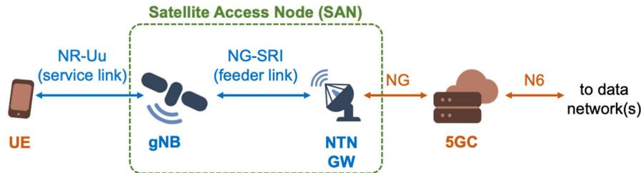
Figure 6: NTN architecture with regenerative payload and direct access: full gNB on-board.
