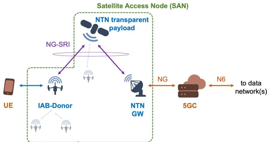
Figure 19: NTN architecture for indirect access with transparent payload: backhaul to the 5GC.
