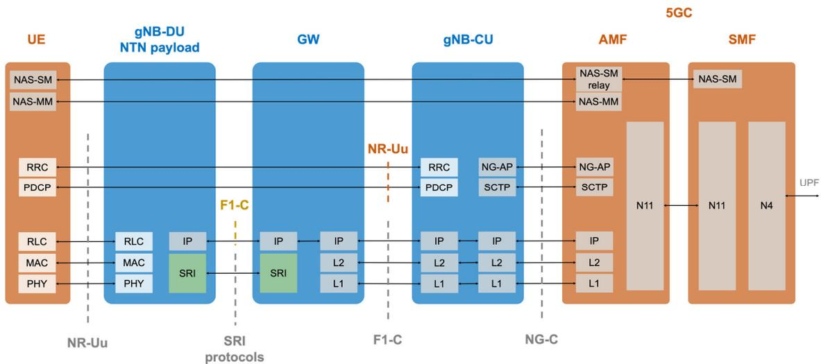
Figure 14: CP protocol stack: regenerative payload with functional split for direct access.
