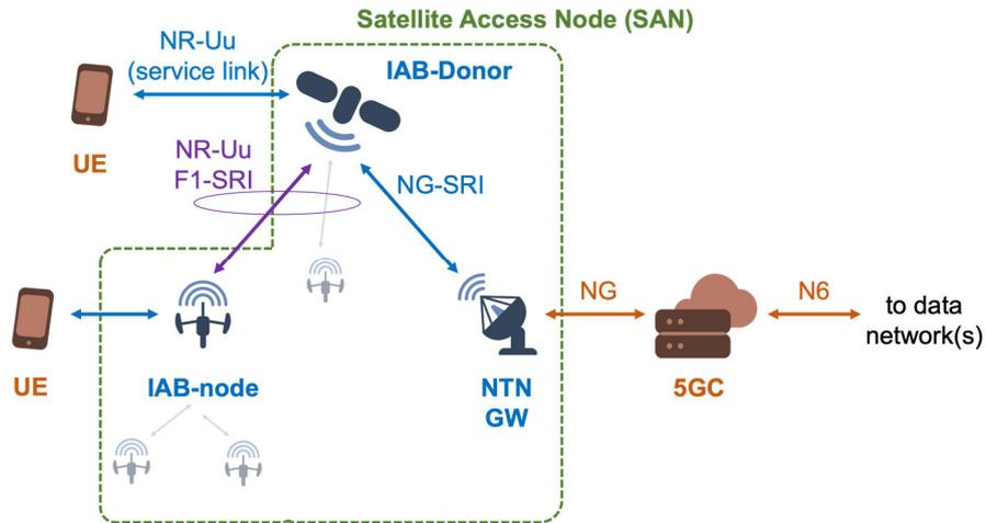
Figure 20: NTN architecture for indirect access with regenerative payload: full IAB-Donor on-board.
