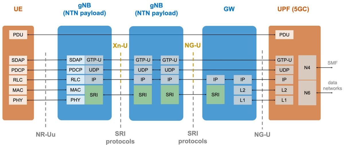
Figure 10: UP protocol stack: regenerative payload and direct access with full gNB on-board and ISL.
