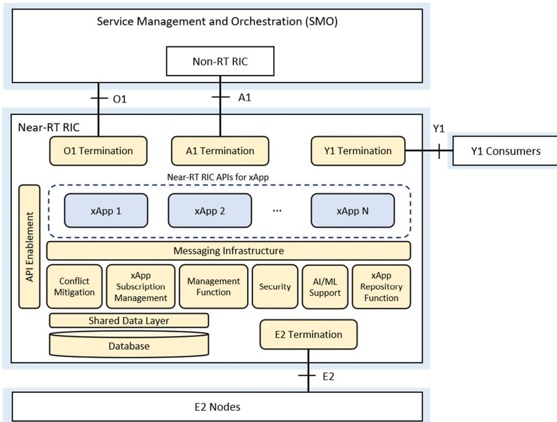
Figure 38: Near-RT RIC Internal Architecture.
