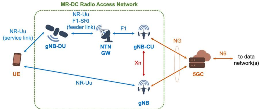
Figure 32: MR-DC architecture between TN and NTN with regenerative payload: gNB-DU on-board.
