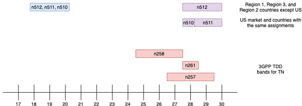
Figure 40: Representation of the currently considered NTN Ka-band allocations in Table 8.
